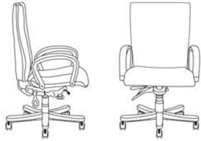
26-UB Management/Conference Chair Inset upholstered hardwood arms, hardwood base and unitized steel underbase. Seat: 21"W 20"D Overall: 25.5"W 25"D 37-40"H
